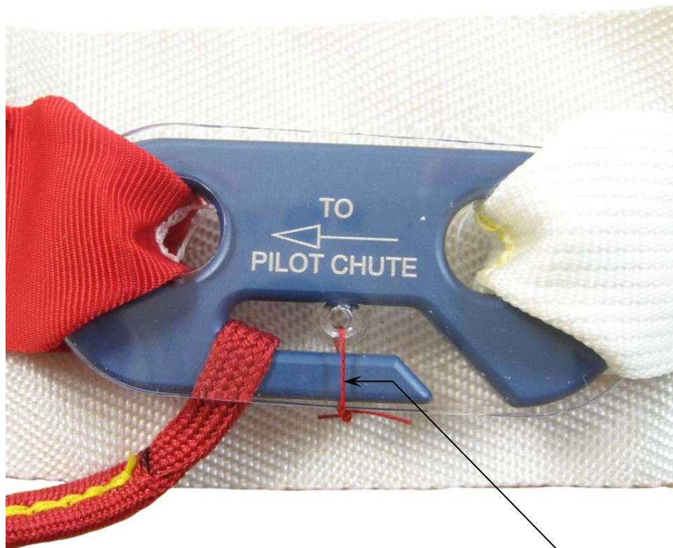
Single pass of red rigger seal thread
