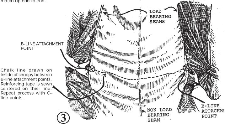
NOTE: When finished, these reinforcement tapes will run spanwise ( from side to side across the canopy ) from line attachment point to line attachment point at the "B" lines and the "C" lines.
