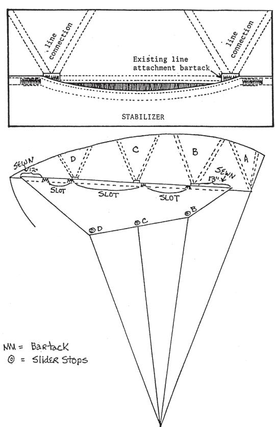
Because it is necessary to disconnect portions of the stabilizers adjacent to the "B" and "C" line attachment point to do this reinforcement, I have included this Diagram of stabilizer configuration.
