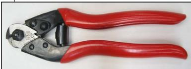
With appropriate cable cutters, snip to the correct length,
