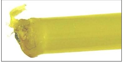
Examples of poorly burned cable ends.
