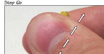
In one smooth and fluent motion, quickly and repeatedly pull the firmly griped cable completely out rotating it 90° each time.
