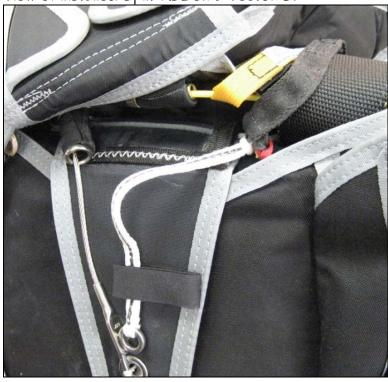
Notice how the left side cutaway cable is in passing ONLY through the Yellow Loop, and the black RSL pin, and Skyhook lanyard larks headed on the end.
