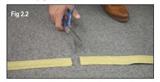
NOTE: Be sure your scissors are very sharp. We suggest you practice on a lower section of Kevlar (below the disc). The cut will be more accurate when the Kevlar is under tension.
