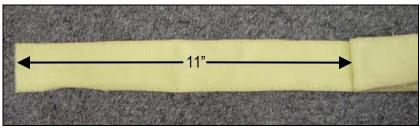
**4.** The two sides of the bridle will now be converted into loop ends. Mark **5"** from each of the two ends on the outer surface (**Fig 4.1**). With inner surface facing up, fold the webbing into the center on this **5"** mark (**Fig 4.2**). Using E-thread, sew a double pass of zigzag stitching, or one bar tack, or four passes with a single needle machine across this mark (**Fig 4.3**).
