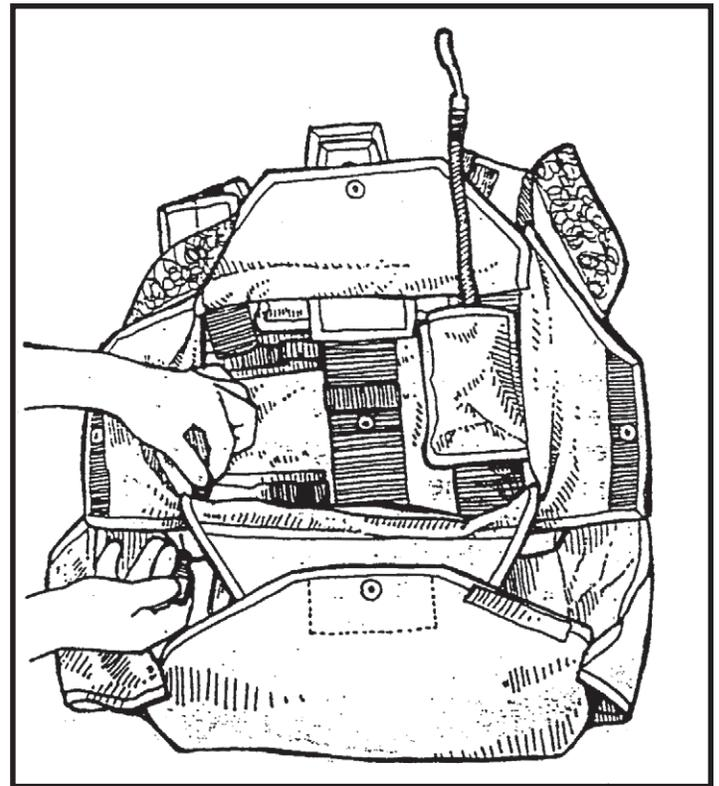
9. Thread the activation unit cable through the channel that runs along the left side of the main pack tray.
