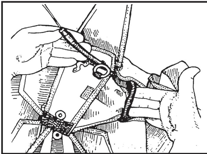
6. Measuring along the center line of the reserve top flap (Flap #6), measure up 4 inches from the center of the grommet and mark. This mark indicates the lower edge of the mounting bracket.
