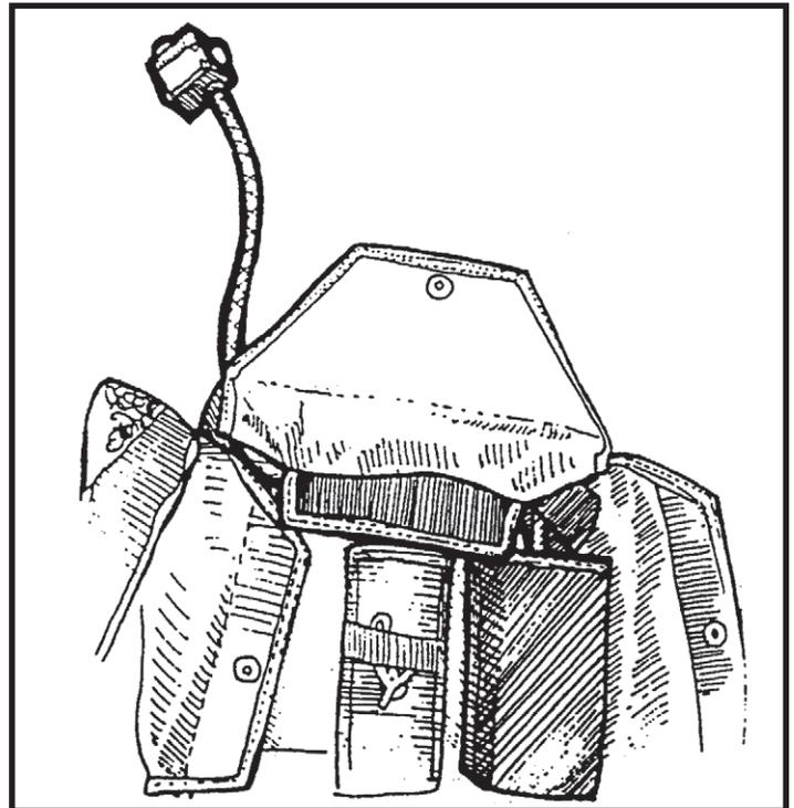
10. Route the sensing unit cable under the Velcro flap on the left hand shoulder yoke.
