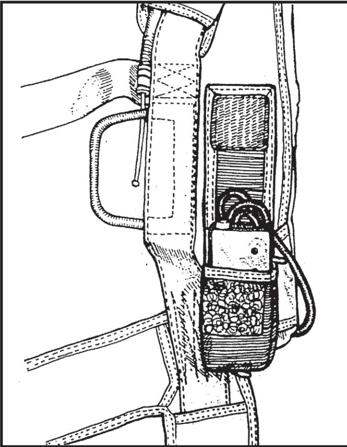
12. Secure the sensing unit into the pouch with a piece of Type 3 sheathing by passing one end through the grommet in the bottom. of the pouch, through the hole in the bottom of the unit and back out the grommet. Then pass a small metal washer over both ends of the Type 3, snug it up and tie an overhand knot. Cut off the excess Type 3 and sear the ends.
