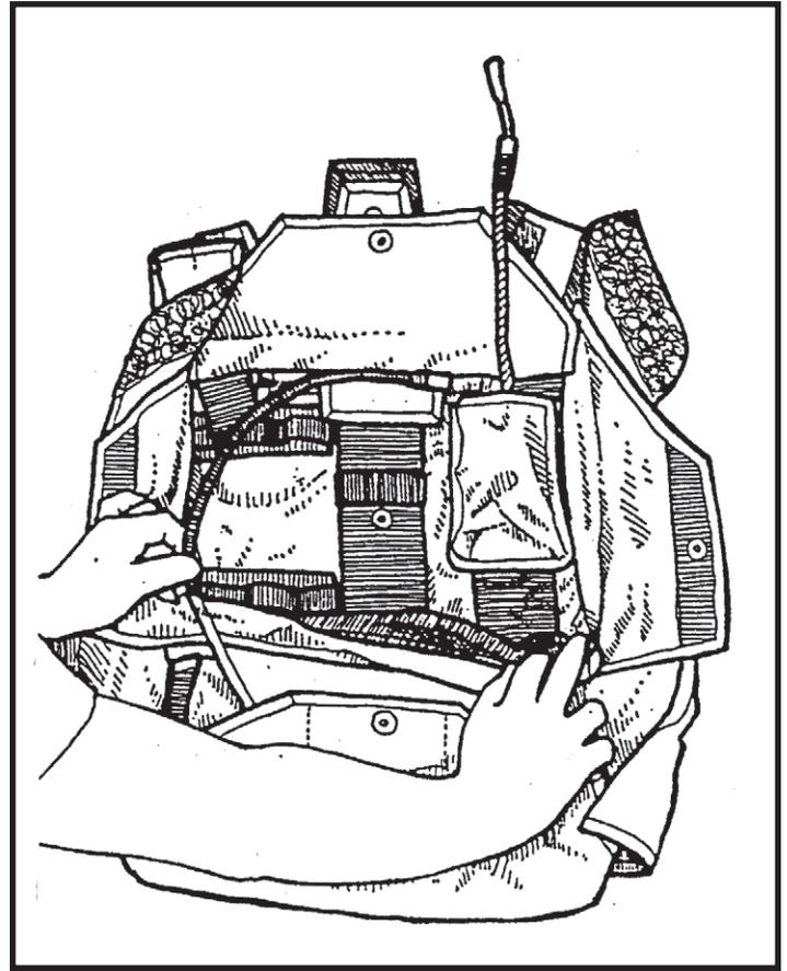
6. Pull the cable gently to seat the unit in the pouch and remove any slack in the cable.
