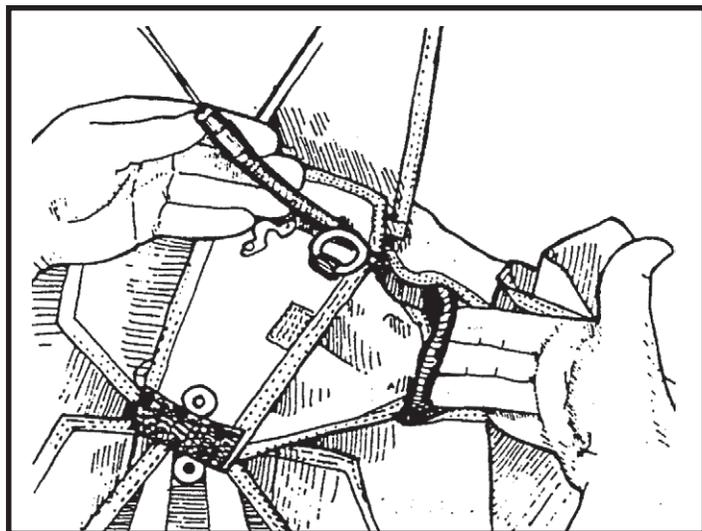
11. Using the pouch provided, mount the sensing unit to the diagonal strap. Coil the a cable and tuck it into the pouch.
