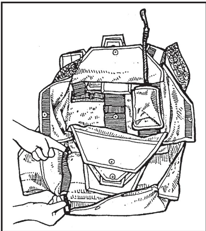
10. Route the activation unit cable through the hole in the lower left hand corner of the main container. Attach the activation unit cable you have just threaded to the sensing unit cable.
