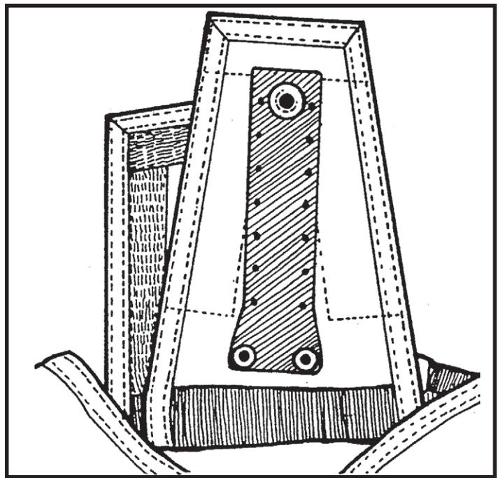
5. Thread the activation unit cable through the long thin Pin Puller pouch on the right side of reserve pack tray and out the bottom. Slide , activation unit into the pouch.
