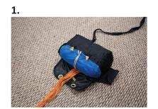
Insert the prepared canopy into the main deployment bag.
