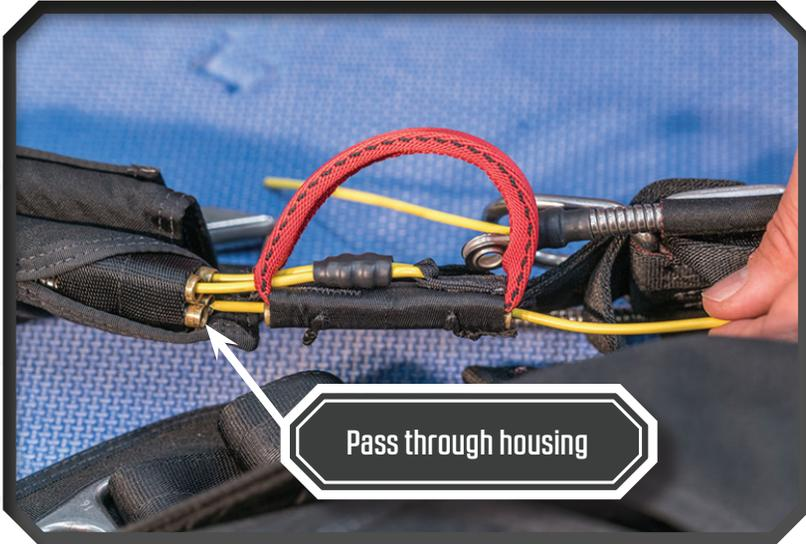
Install the sloop mode release cable through the housing which is part of the Red Cutaway Handle.
