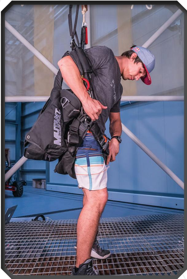
Get into the harness and begin adjusting as seen in the following photos. It's important to understand that the leg straps do not need to be as tight as normally seen on a conventional Vector. This will improve the comfort when in flight mode.
