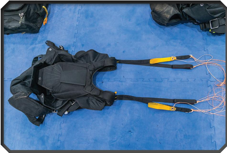
Setup the main risers using the canopy you will jump in the beginning. It's recommended that you start off with a more lightly loaded and less aggressive wing than what you normally use.
