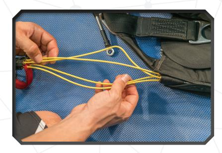
All cables should be properly lubricated with silicon.
