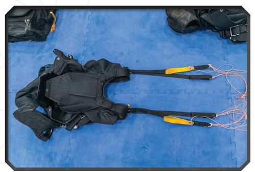
Setup the main risers using the canopy you will jump in the beginning. It's recommended that you start off with a more lightly loaded and less aggressive wing than what you normaly use.
