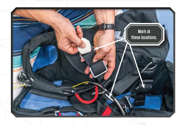
Once in the harness with leg straps and chest strap adjusted, the belly band can't be adjusted. First, close the seat belt adapter. If the belly band is too tight or too loose, undo it and adjust the 3-bar adapters accordingly. Do the seat belt clips up again and check the adjustment. Once the belly band is set, it should not need further adjustment. The fitting of the belly band will change slightly with the main container packed.
