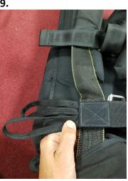
Place webbing side of belly band on right side of the container at the lower junction aligned with the stabilizer.
