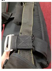
Pass upper loop around the back side of the main lift web.
