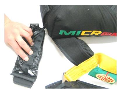
**8.** Stand rig on its side and insert the pilot chute into the pouch until only the handle is exposed.
