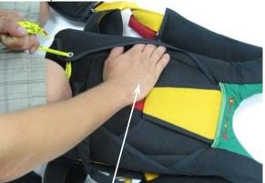
Drawing the side flaps closed may push the internal riser covers out and require being pushed back in while drawing closed.
