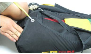
**5.** Insert the closing pin (located on the bridle) through the closing loop from right to left.  $\downarrow$
