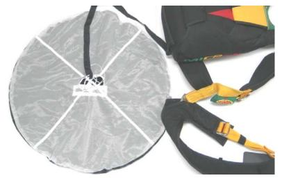
**2.** Fold the pilot chute in half over the bridle.
