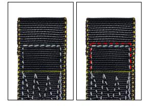
Unpick the ¾ box stitching, with caution not to damage or pull out any part of the webbing
