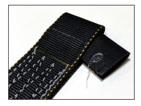
Fold in sides of reserve riser end to allow installation of #6 Rapide link
