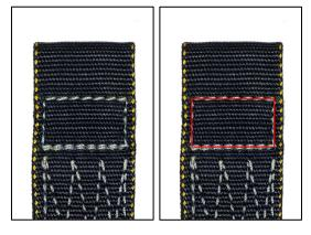
Verify that no webbing is damaged and the 4-point is intact
