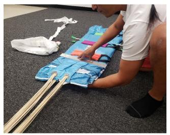
Perform the first S-fold, while controlling the slider grommets and line tension. Using packing paddles will greatly help this.
