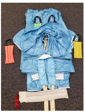
Move to the opposite side and repeat the steps for nose, A/B/C/D, and tail. Dress up and quarter the slider into the folds of B and C, without exposing too much on the front or back. Make sure the line channel in the center of the pack job is clear, and all lines and attachment points are in the center of the pack.
