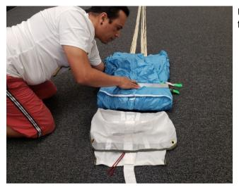
Use a packing paddle to establish the fold line for the remaining S-fold.
