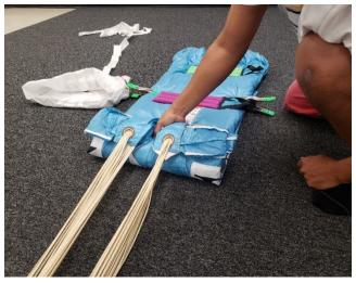
Once first S-fold is complete, the slider grommets should be placed approx. 1" behind fold line.
