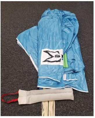
Starting at one side of the canopy, carefully lift the folds of material back towards the center of the pack job until the nose is exposed. Use packing weights hold the opposite side in place. Flake the 4 nose cells to the outside and lay them flat. Use a packing weight to hold them in place.
