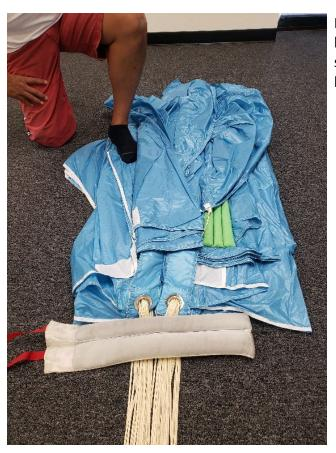
Repeat the previous steps to flake the material between the B and C lines. Repeat the previous steps to flake the material between the C and D lines.
