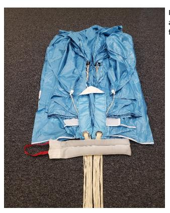
Place a packing weight at the base of the canopy and maintain line tension. Dress up the canopy folds from flaking, keeping the lines centered.
