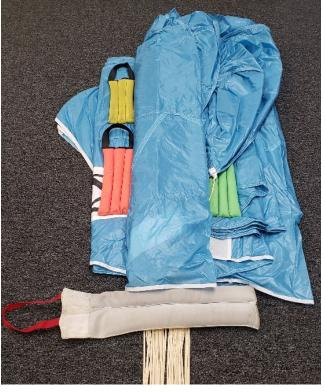
Smooth out the fold between the A and B lines and create a reduction fold in half towards the center of the pack job. Go to, but do not go beyond the line attachment points. Use weights to control the fabric and folds.
