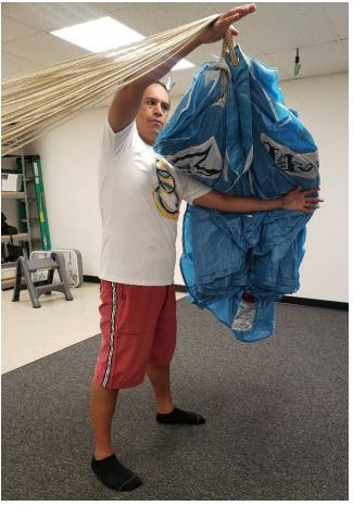
Hold the lines in one hand with tension forward and use your free arm to support the canopy fabric while gently placing the canopy on the packing surface.
