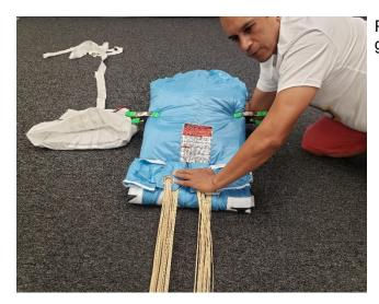
Press down and hold tension on lines and slider grommets in place.
