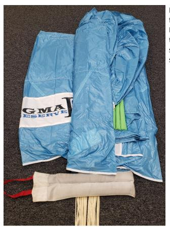
Flake the material between the A and B lines away from the line channel in the center of the pack job. Be sure to have A and B line attachment points and their reinforcement tapes in the center of the pack, stacked together. Even up the bottom seams at the stabilizer.
