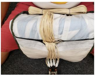
Stow the remainder of the suspension lines into the pouch on the underside of the bag using S-folds that extend completely from one side of the pouch to the other. Close the two Velcro tabs mating. Be sure none of the lines are trapped between the hook and loop fastener at the mouth of the pouch.
