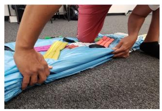
When the nose folds are complete, the leading edge should be even with the edge of the cocooned canopy.
