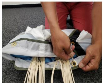
Tuck side flap of bag inwards neatly enclosing the corner of the canopy and pass the safety stow through the smooth face of the bottom grommet.
