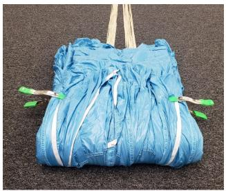
Reach under cocooned canopy to fold over second S-fold.
