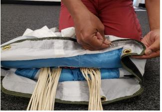
Turn the grommet inward such that the safety stow will pass through the smooth face of the grommet
