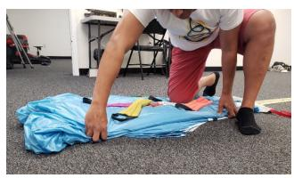
Place this in between the A/B folds and B/C folds, effectively cocooning the fabric from C lines until the tail.
