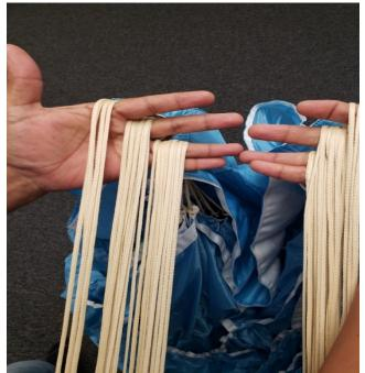
Prior to packing, inspect canopy for any damage, and ensure correct line continuity.
