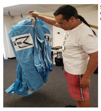
Spread the nose of the canopy with an even number of cells to the left and the right, leaving the center cell fully exposed in the middle.
