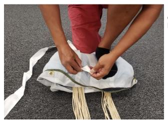
Use a needle fold of bridle material to secure one end of the safety stow allowing you make the first locking stow.
