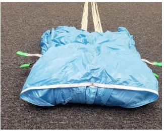
Ensure that nose folds are still rolled up and placed close to center. Dress center cell to the width of the pack job, covering the nose folds on each side.
