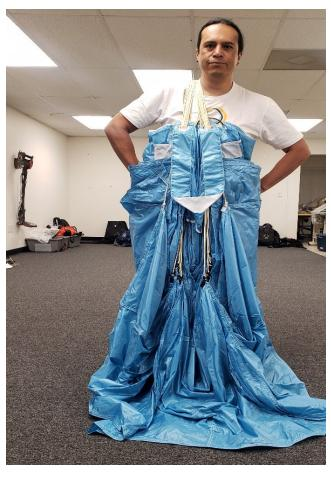
Place canopy over shoulder, and flake the nose counting each cell. When you have the entire nose flaked, tuck it between your knees and hold it there. Clear the stabilizers. Flake each side outwards, with lines and line attachment points placed in center. Quarter the slider. Clear the tail, flake the material between each steering line outwards, with lines and line attachment points placed in center.
