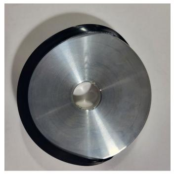
Continue gently heating the edge of the disk cover as you work it around the drogue disk with the LB Tool.
