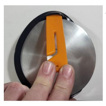
Use LB Tool to work warmed area of disc cover over the edge of the disk.
