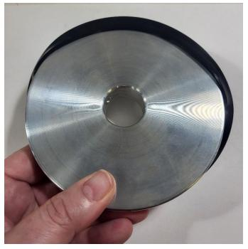
Heat disk with the low setting of a heat gun or hair dryer to soften plastic.
