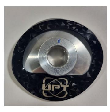
Align Disk cover with drogue disk. Horizontal edge of disk should be perpendicular to arrow.
