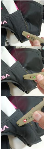
Place a magnetic polarity tester on top of the closest magnet in the yoke flap. The polarity should be North.
