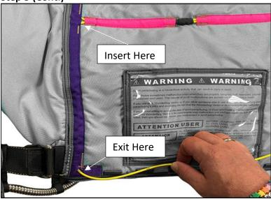
The longer cable is installed and directed toward the lower part of the back pad.
