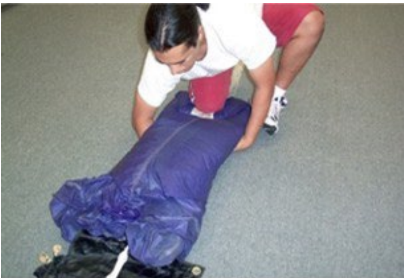
Reach underneath canopy in preparation for the second S-fold.
